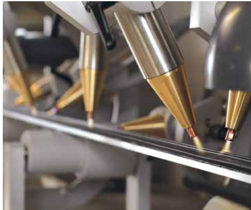
**Two common applications for pre-treatment of automotive EPDM profiles with plasma are prior to flocking and slip-coating. In the flocking process, treatment is necessary to achieve a strong bond between the rubber and the adhesive used to attach the flock. For slip-coating it is necessary to treat prior to the spray process to achieve good wettability and optimum adhesion properties of the coating.**
