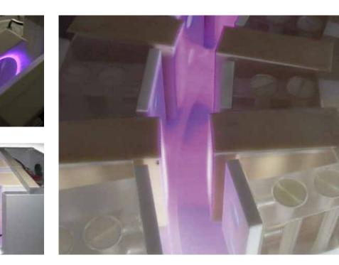
SyrinTEC is specially designed for 360° treatment of PP and PE syringe barrels. Normally the SyrinTEC is built into the printing line and positioned as the final process before the barrels enter into the printing machine. Using the SyrinTEC enables treatment of the entire outside surface without any inside treatment, which would increase friction on the inside barrel and cause the plunger to drag when used.
